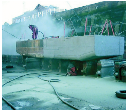
Grit blasting trials underway at Dunstons Ship Repair in Hull UK.
